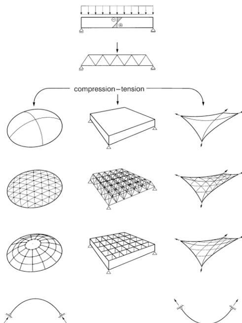
Fig. 4: The evolution of lightweight spatial structures
