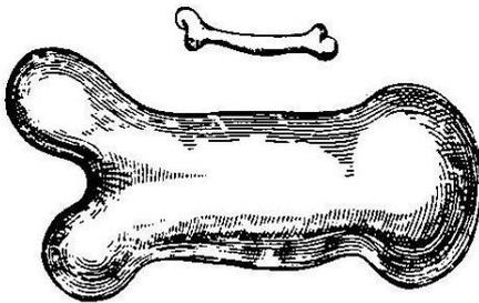
Fig. 1: Galilei's demonstration of the scale effect
