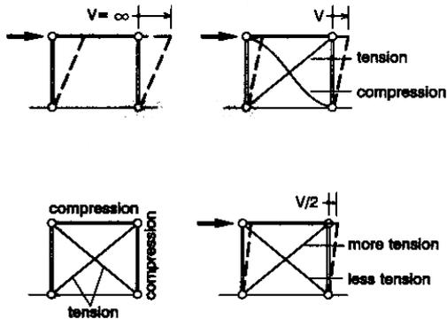
Fig. 3: The principle of prestress (Top left: unstiffened kinematic system; Top right: The diagonal in compression becomes slack and only the diagonal in tension is active; Bottom left: prestress: before loading the diagonals are shortened i.e. pretensioned; Bottom right: in a prestressed system both diagonals share the load)
